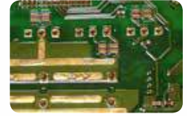
Enhanced conformal coating
